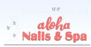
FABRICATE AND INSTALL ONE SET OF 5" DEPTH INTERNALLY ILLUMINATED CHAN, LTRS. 3/16" THICK #2283 RED PLEXIGLAS FACE WITH 1" BLACK JEWELITE TRIMCAP. -. 063 ALUMINUM PRE PAINTED BAKE BLACK RETURNS. INTERIOR SIDE WALL AND BACKS OF LETTERS WILL BE WHITE. WHITE LED FOR ILLUMINATION. 2"x12" .063 ALUMINUM WIREWAY PAINTED TO MATCH WALL. ALL U.L. LISTED COMPONENTS.
