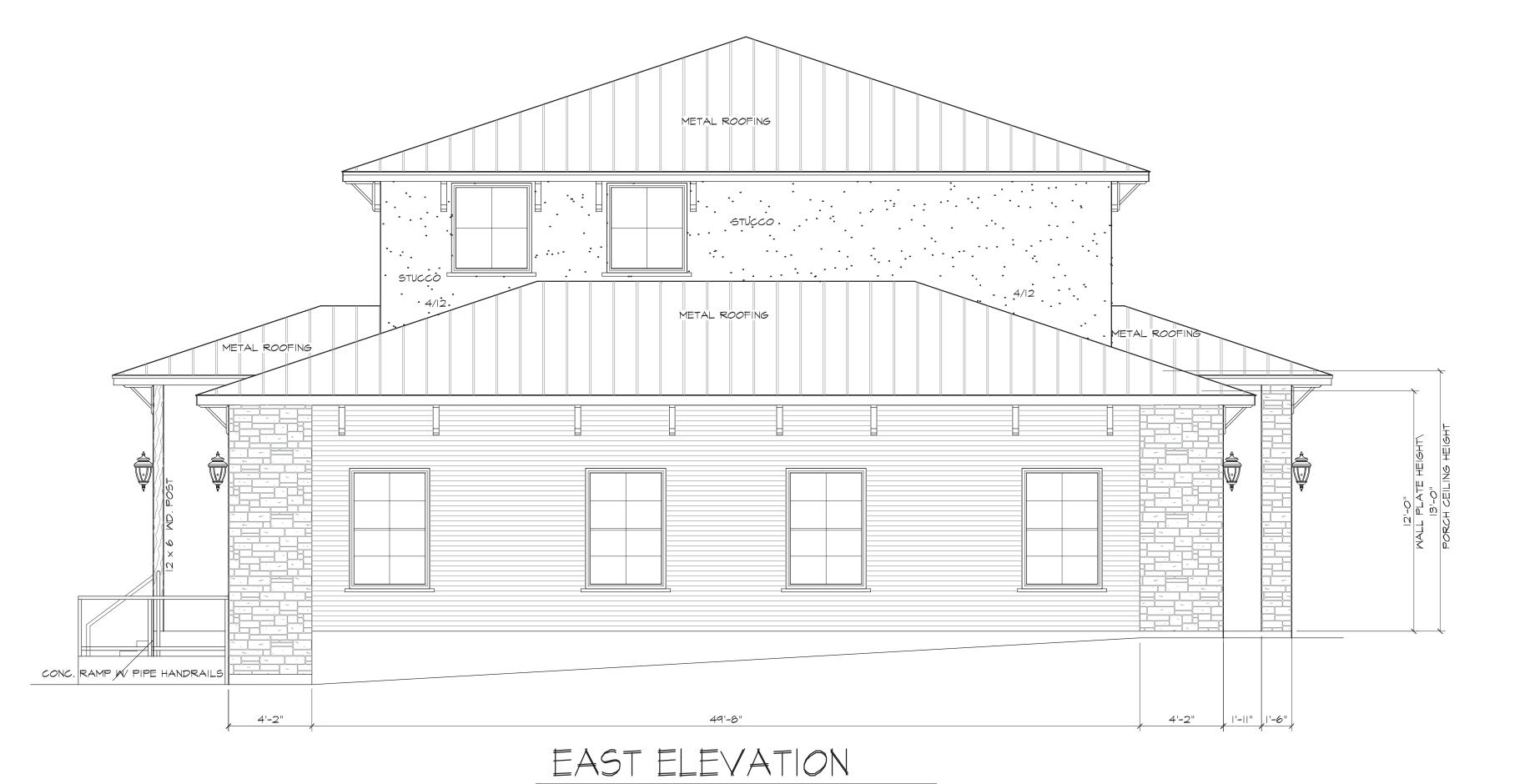
COLOR AND MATERIAL WILL BE COMPATIBLE WITH THE OTHER BUILDINGS WITHIN THE PLANNED DEVELOPMENT. FIRST FLOOR ELEVATION IS 100% MASONRY
