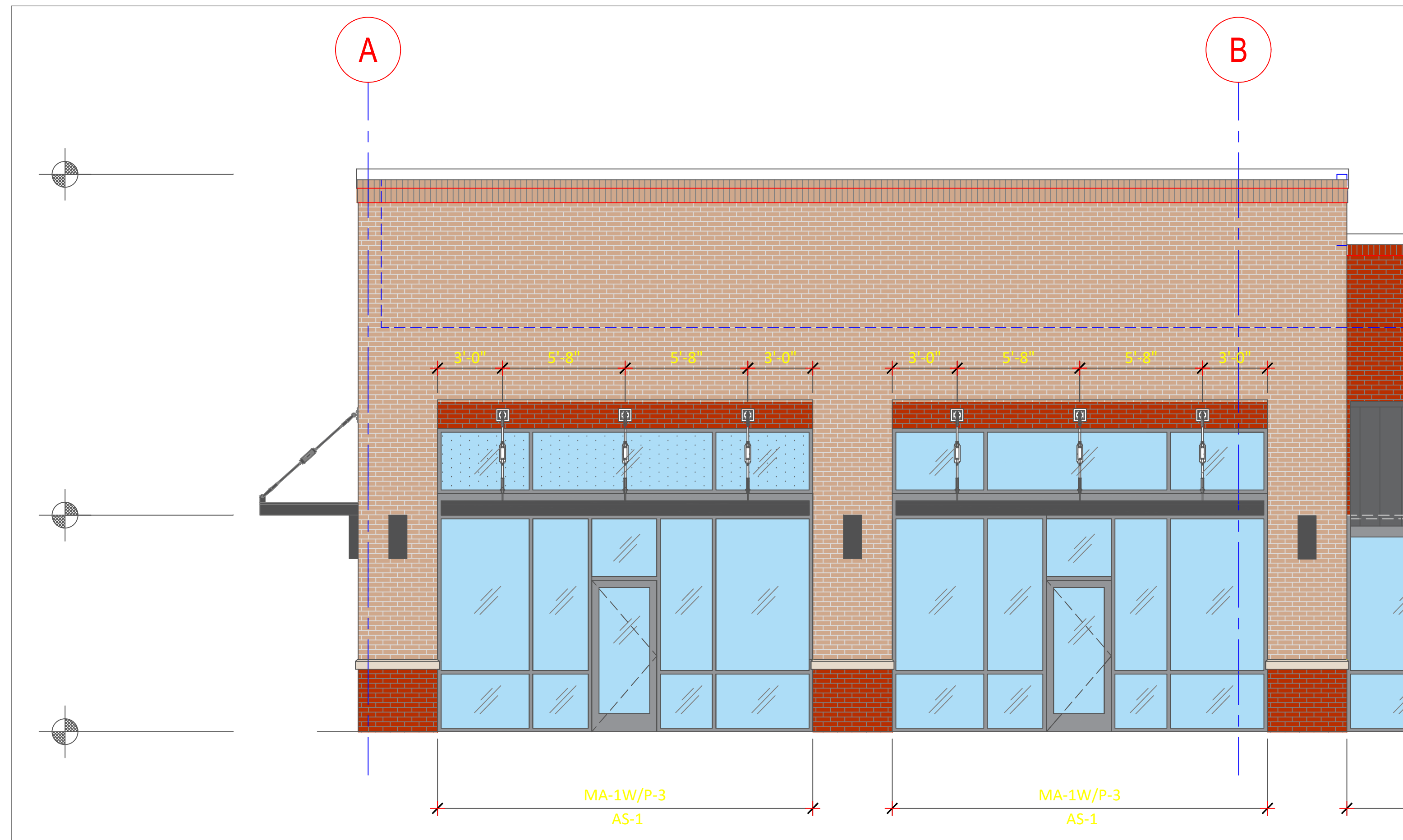
1 SOUTH ELEVATION - EXISTING STOREFRONT SCALE: 1/4" = 1'-0"
