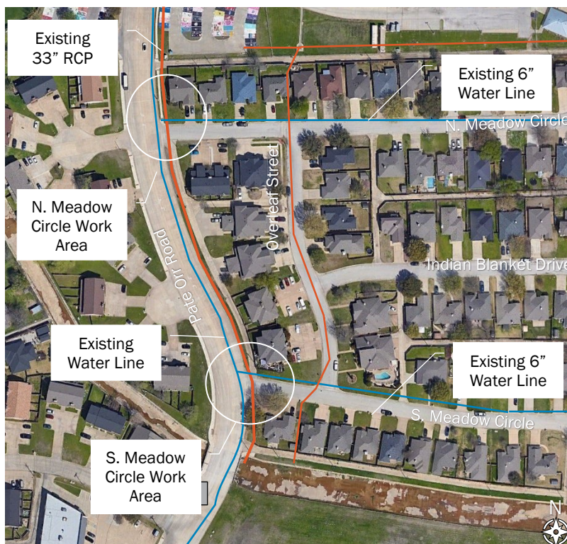
Figure 3: Water line lowering and stormwater replacement in Bluebonnet Hills neighborhood at the intersections of N. Meadow Circle and Pate Orr Road and S. Meadow Circle and Pate Orr Road
