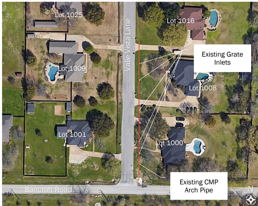
Figure 4: Existing CMP arch pipe along Valle Vista Lane to be shown on construction plans.
