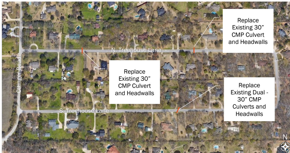
Figure 5: Approximate locations of culvert replacements along N. Treehouse Lane and S. Treehouse Lane.
