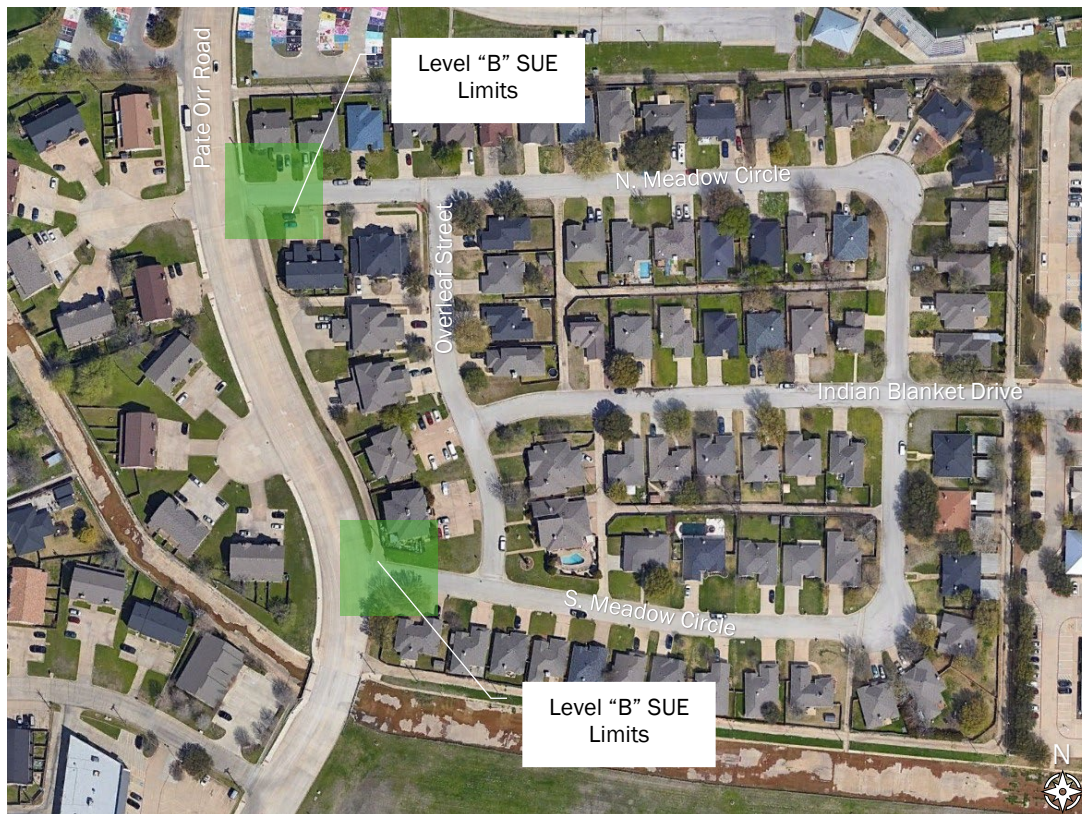
Figure 6: Limits of Level “B” SUE for the water line lowering and stormwater replacement in Bluebonnet Hills neighborhood at the intersections of N. Meadow Circle and Pate Orr Road and S. Meadow Circle and Pate Orr Road
