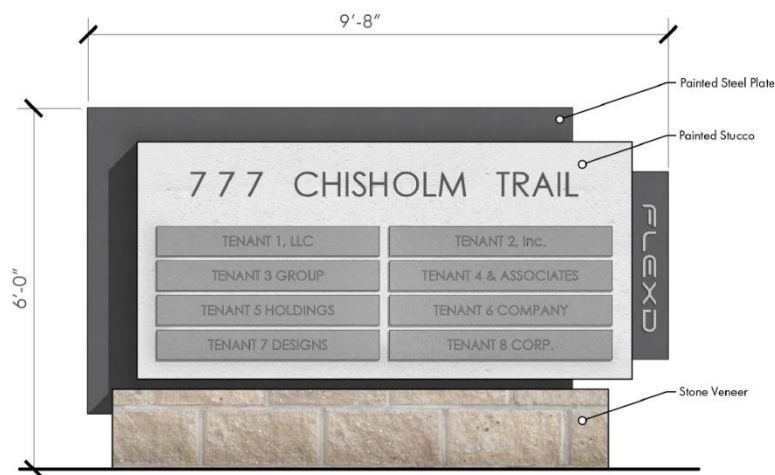
TYPICAL MONUMENT SIGN ELEVATION
