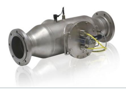
The UV system works cleanly and with efficient use of energy, based on continuously variable medium pressure lamps, and can therefore automatically compensate for variations in the water quality or level of contamination.
