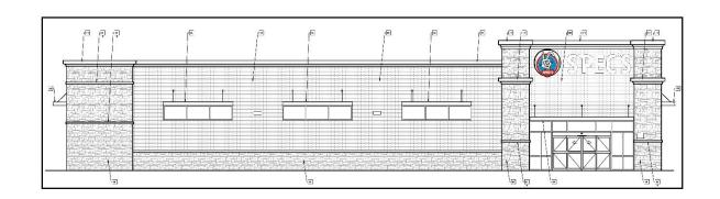
The Applicant proposes to construct the entire 12,180-square-foot single-story building with brick and stone, exceeding Town Center (TC) guidelines of 75% brick, stone, or cast stone.
