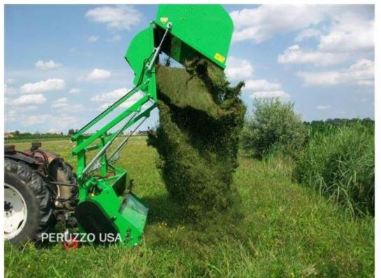
Panther 1800PRO 72" Flail Collection Mower: 64cu' Cap, Hyd High Dump VertiCutting Capable
