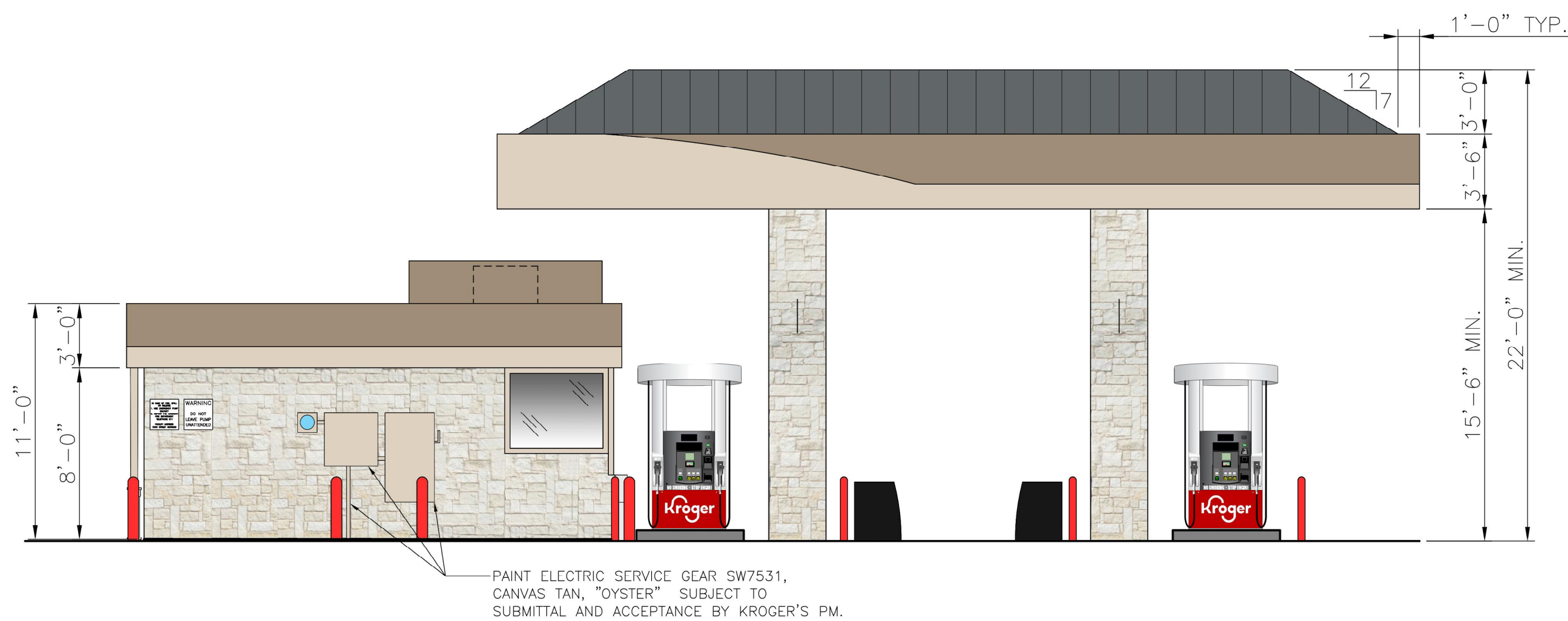
2 FUELING CENTER LEFT (SOUTH) ELEVATION SCALE: 3/16"=1'-0"
