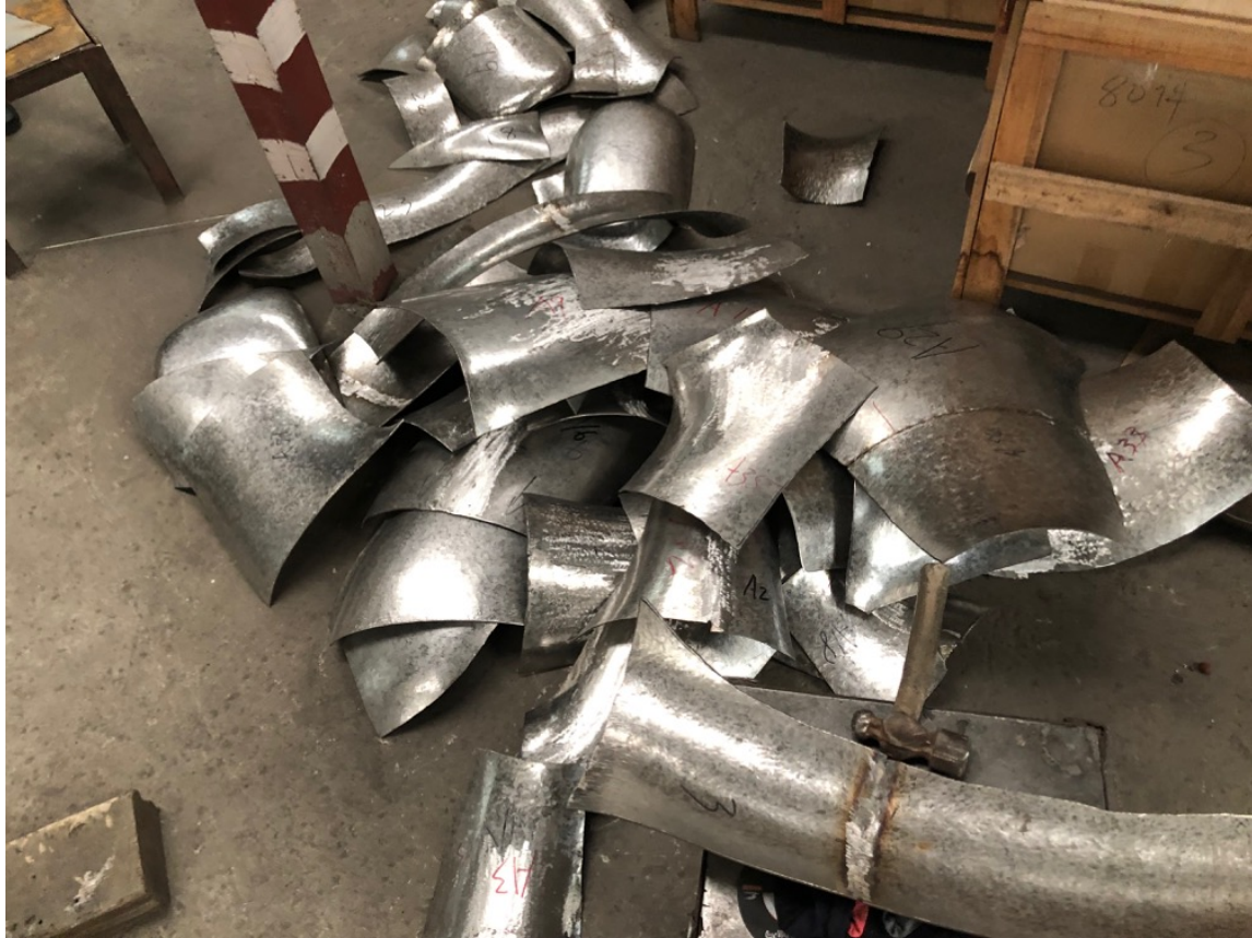
Stainless steel material cut and shaped to the fiberglass puppy figure.
