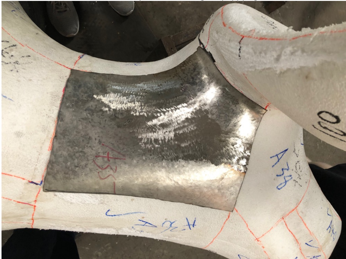
Stainless steel material cut and shaped to the fiberglass puppy figure.
