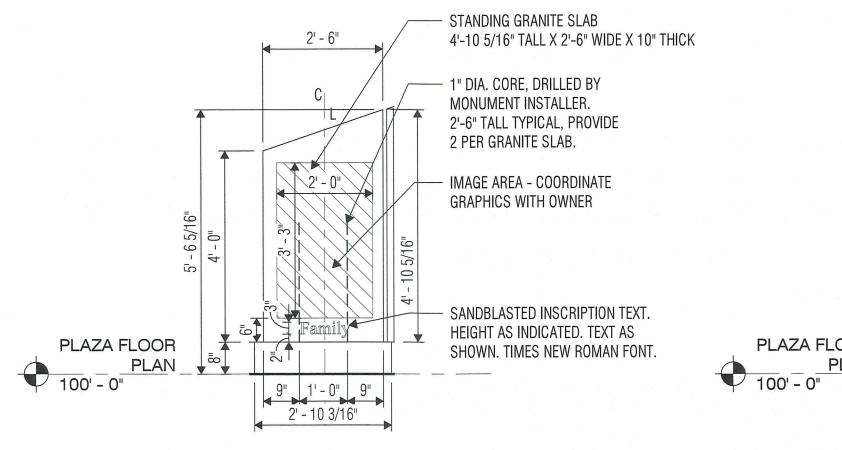
ELEVATION NORTH - PANEL B SCALE: 1/2" = 1'-0"
