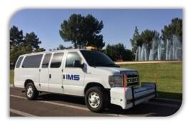
update with integration into Lucity. IMS will survey approximately 252 test miles as we will perform two passes on the arterial and collector roadway network. The IMS approach to pavement data collection allows for detailed coverage of residential roadways with just a single pass. IMS collects all pavement distress data in accordance with a modified version of the ASTM D6433 data collection protocols.
