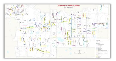
street rehabilitation plans or most of the data in the pavement management program. An output of the PCI score for each segment is illustrated in the adjacent image.
