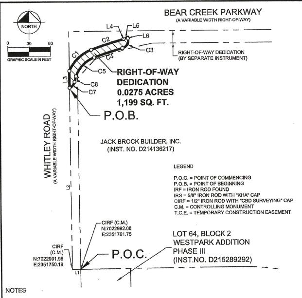
Bearing system based on the Texas Coordinate System of 1983(2011 adjustment), North Central Zone (4202) with an applied combined scale factor of 1.00012. A metes & bounds description of even survey date herewith accompanies this survey plat.
