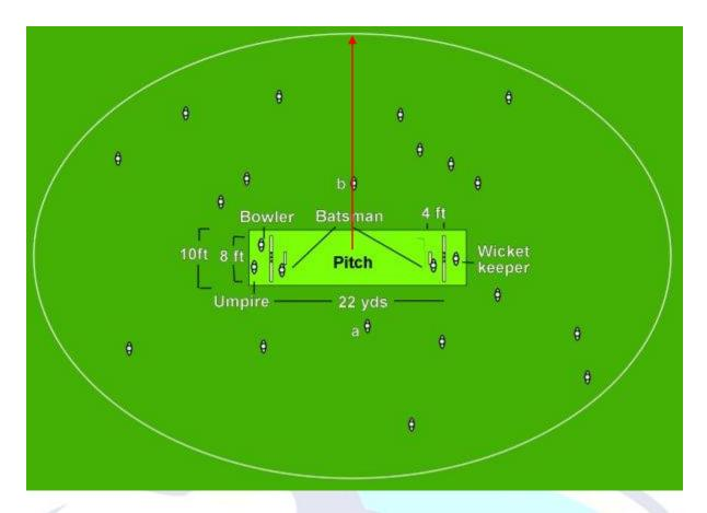
Note: Red arrow (above) showing the radius of circle measured from the center of the pitch. The radius is 75 yards or 225 feet.
