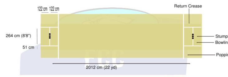
The actual dimensions of the pitch are 66 feet by 8 feet & 8 inches. However in view of minimizing the maintenance, the concrete slab is laid on a slightly larger area such as 90 feet by 10 feet.
