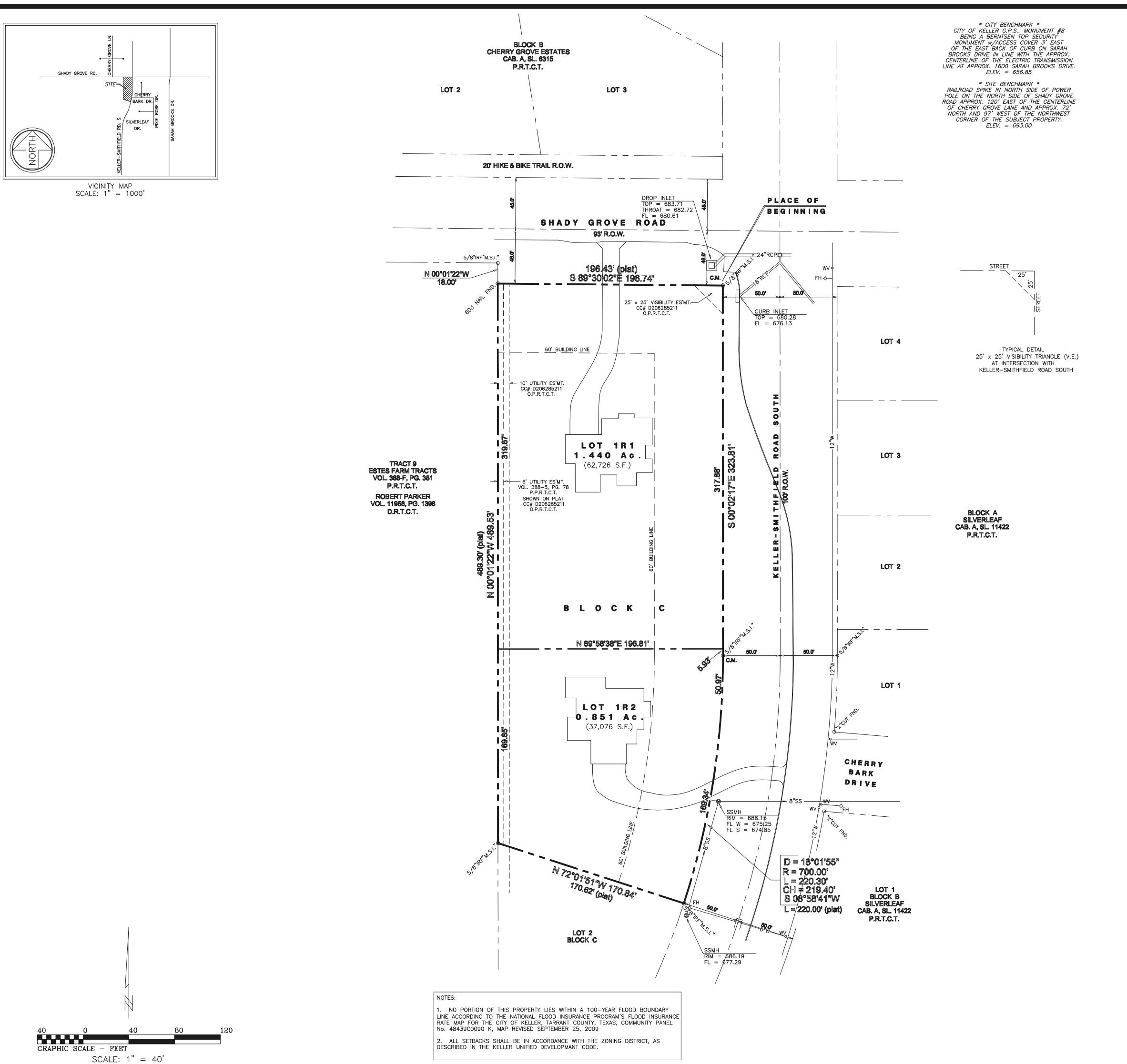
BASIS OF BEARINGS: WEST RIGHT-OF-WAY LINE OF KELLER-SMITHFIELD ROAD SOUTH AS SHOWN ON PLAT RECORDED IN CABINET A, SLIDE 11422, P.R.T.C.T.
