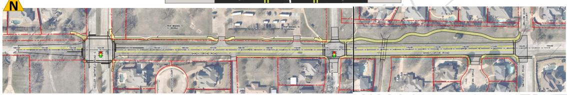
Convert a two-lane, bar ditch street to a three-lane street with curb & gutter and sidewalks ~0.3 miles in length
