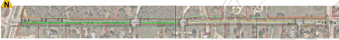
Convert a two-lane, bar ditch street to a four- to five-lane roadway with curb & gutter and sidewalks ~0.65 miles in length
