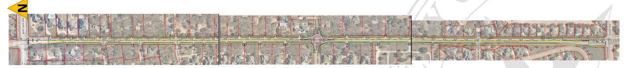
Convert a two-lane, bar ditch roadway to a three-lane roadway with curb & gutter and sidewalks. Bicycle accommodation and intersection control at Bancroft TBD.
