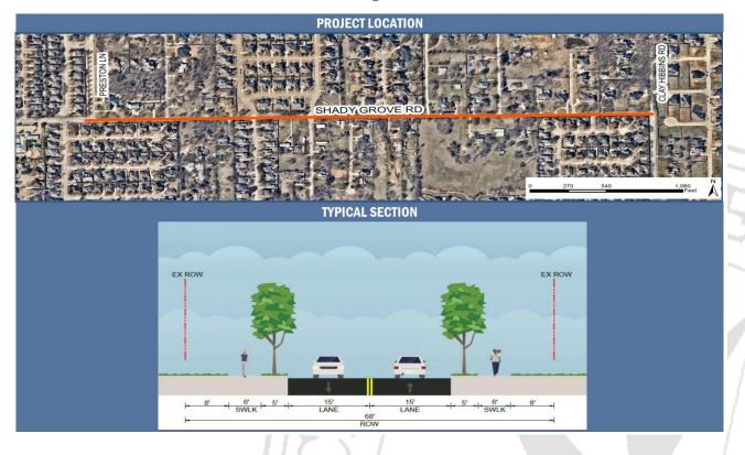
Convert a two-lane, bar ditch street to a two to three-lane roadway with curb & gutter and sidewalks. North Richland Hills would take the lead.
