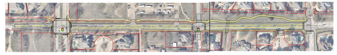
Convert a 2 lane, rural bar ditch to an urban 3 lane, curb & gutter with sidewalks
